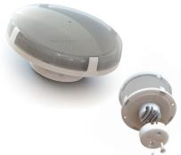
It has a diameter of 60 mm and its base can be equipped with 10 or 20 LEDs according to the power level you want to obtain. It is available in all the three operative modes (Plug & Play, Controllable Pixel and Controllable SMART) and in both the Direct Wire and Frontal Pull Out installation systems.
