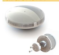
It has a diameter of 75 mm and its base can be equipped with 20 or 30 LEDs according to the power level you want to obtain. It is available in all the three operative modes (Plug & Play, Controllable Pixel and Controllable SMART) and in both the Direct Wire and Frontal Pull Out installation systems.
